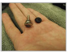
Using the Phillips 2 Screwdriver, remove the 1 1/16" strap button screws and felt washers from both ends of the body.
