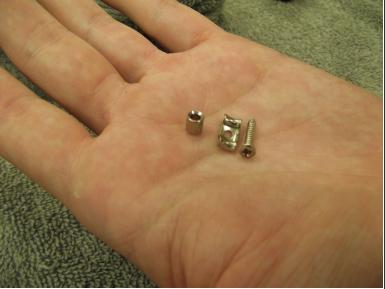
Using the Phillips 2 Screwdriver, unscrew the 9/16" screws from each of the two spring trees and remove the trees and spacers.
